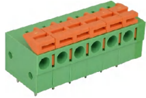
SAHO508 Pitch 5.08mm Poles 1p~24p PCB spring-cage terminal blocks, horizontal wire inlet
