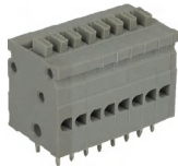
SDVD250 Pitch 2.5mm Poles 1p~16p PCB spring-cage terminal blocks, vertical wire inlet
