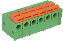
SAHO500 Pitch 5.0mm Poles 1p~24p PCB spring-cage terminal blocks, horizontal wire inlet
