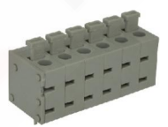
SPVO500 Pitch 5.0mm Poles 2p~24p PCB spring-cage terminal blocks, vertical wire inlet
