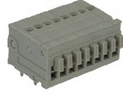
SDHD254 Pitch 2.54mm Poles 1p~16p PCB spring-cage terminal blocks, horizontal wire inlet
